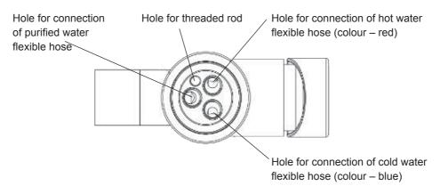
Figure 2. Flexible hoses and threaded rod connecting
