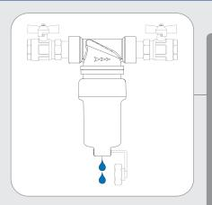
**FDM-2** must be always installed in the upright position. It is recommended the installation of shut-off valves before and after FDM-2.
